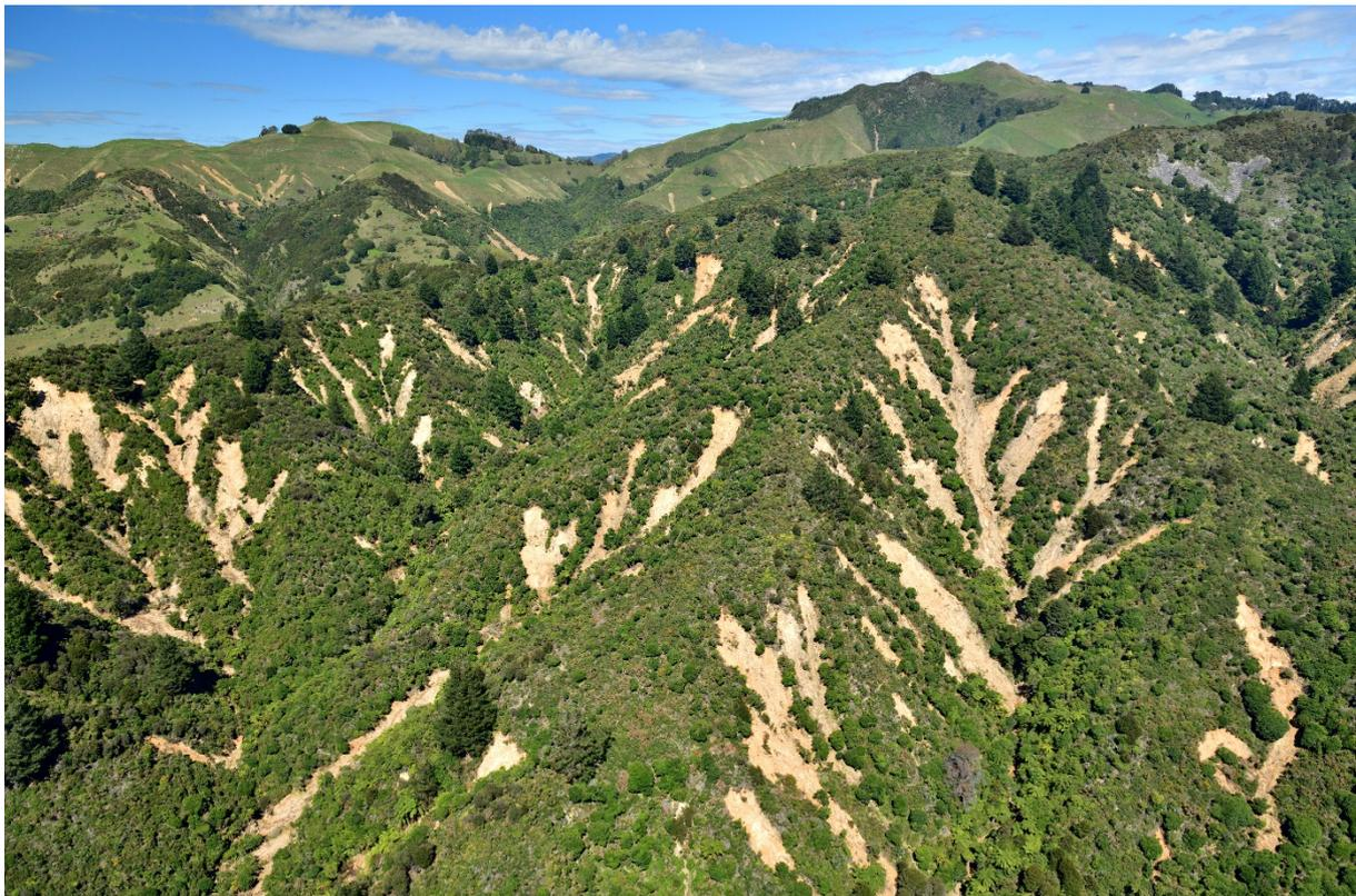
Figure 2.7 Shallow debris flows initiated in soil or colluvium in gully heads in the Otuwhero River catchment.
