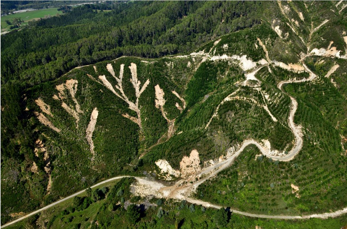
Figure 2.15 Multiple coalesced landslides adjacent to the Marahau River that did not produce significant debris flow runout.
