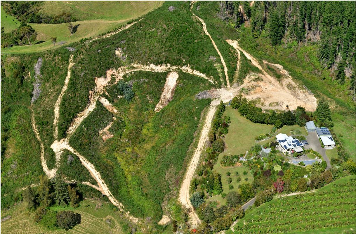
Figure 2.11 Shallow debris flows initiated in soil or colluvium in gully heads in the Brooklyn Stream catchment, near Brooklyn. Several debris flows initiated from forestry roads or skid platforms.
