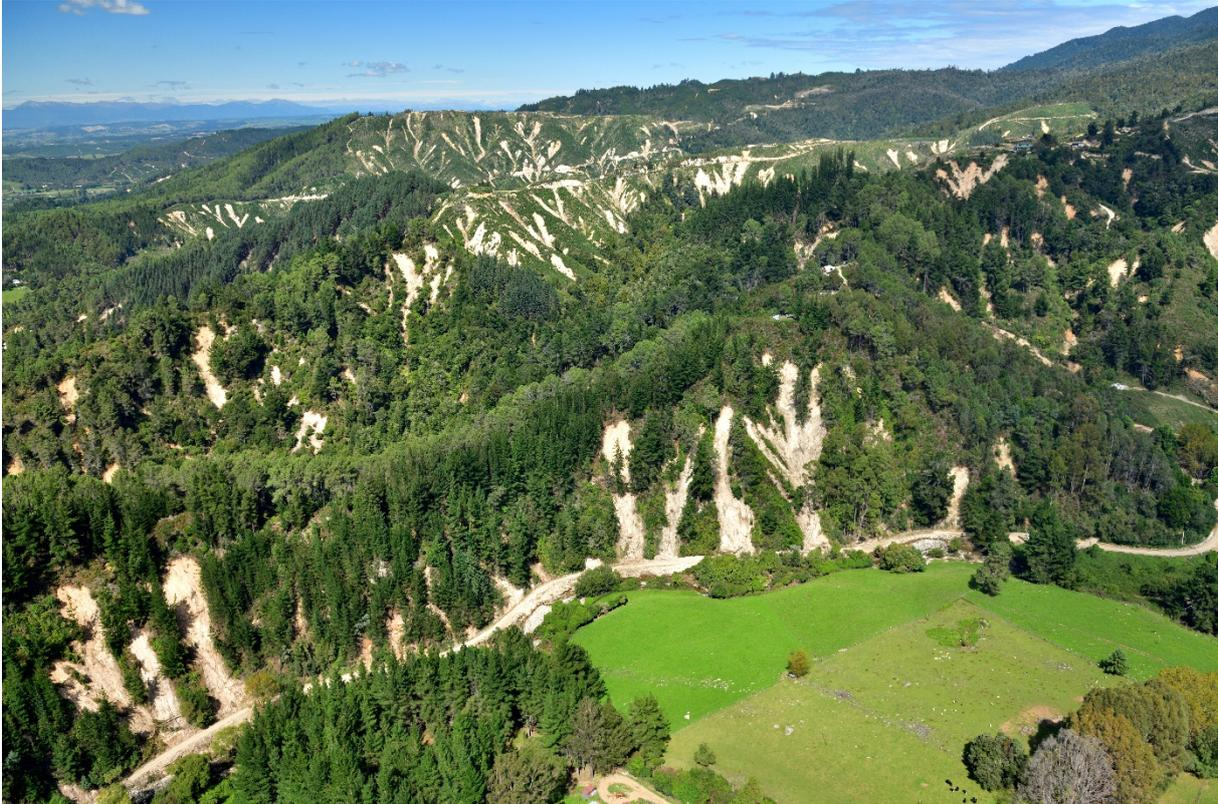
Figure 2.9 Shallow debris flows initiated in soil or colluvium in gully heads. Several debris flows initiated from forestry roads or skid platforms (far centre) (tributary of Holyoake Stream, near Kaiteriteri).
