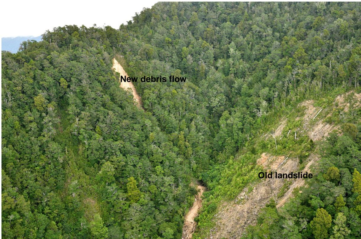
Figure 2.2 Example of shallow debris flows sourced in soil regolith and/or colluvium overlying weathered bedrock. Tributary of Granity Creek, Aorere River. There is also an older landslide scar on the hillslope on the right-hand side.
