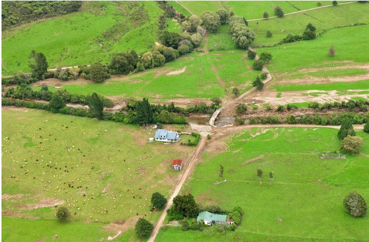
Figure 2.3 Damage to a bridge crossing the Kaituna River, near Aorere, caused by a channelised debris flow. In this location water and entrained debris (mainly trees) built up behind the bridge before spilling out onto the surrounding farm land.
