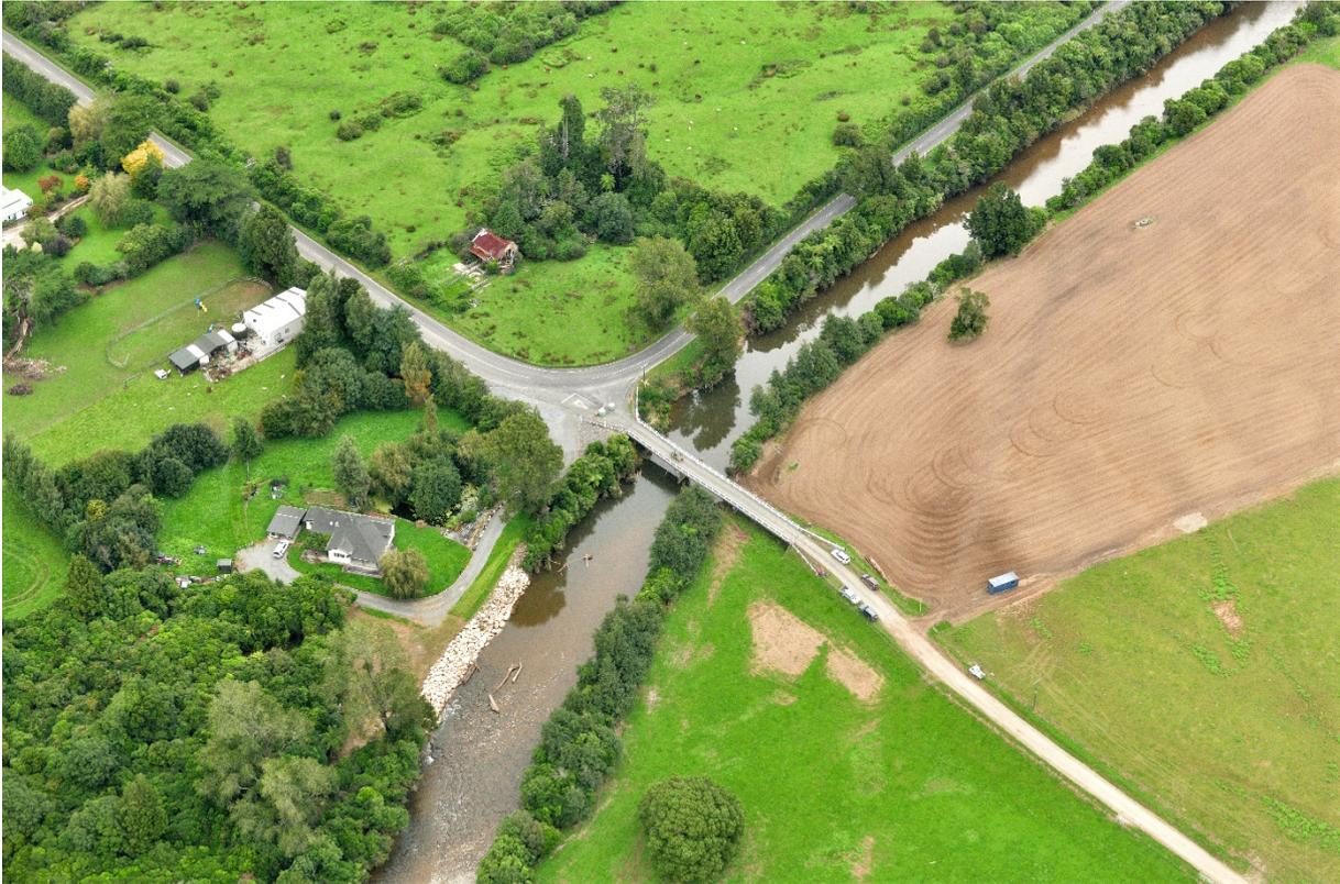
Figure 2.4 Another bridge over the Kaituna River, slightly downstream from of that shown in Figure 2.3, was undermined causing the central section of the bridge to sag.
