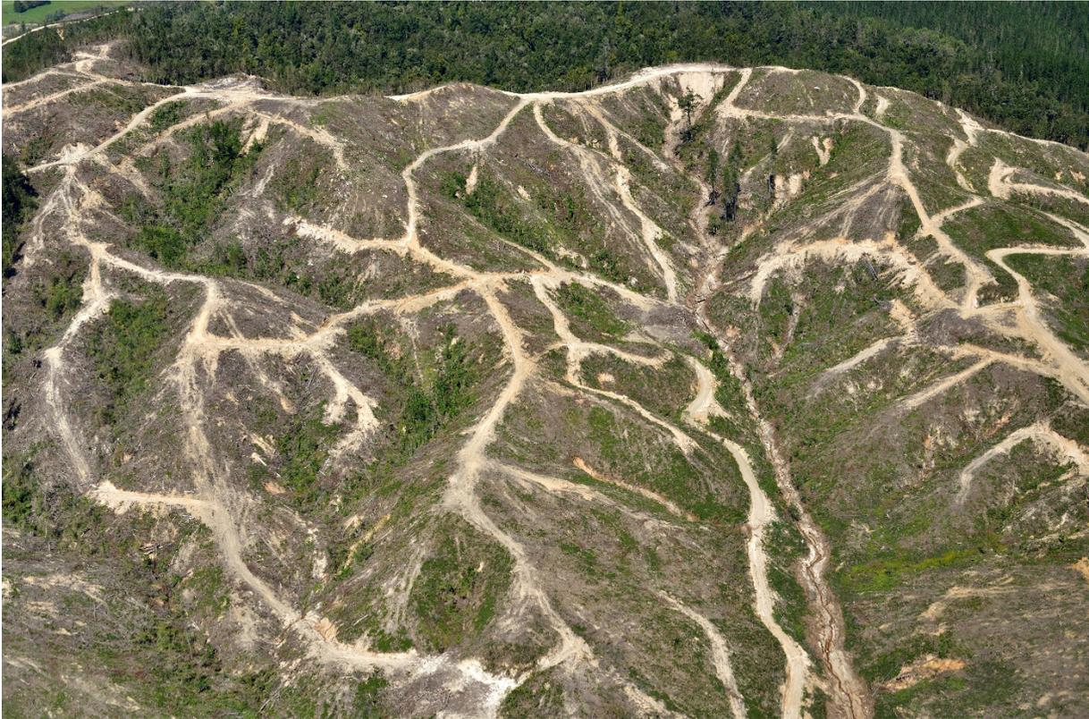
Figure 2.12 Shallow debris flows initiated in soil or colluvium in gully heads in the Waiwhero Creek catchment, near Pangatotara. Several debris flows initiated from forestry roads or skid platforms.
