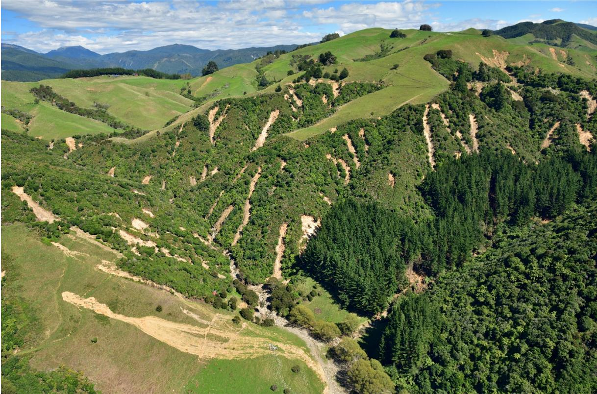
Figure 2.8 Shallow debris flows initiated in soil or colluvium in gully heads in the Atua Stream catchment, near Kaiteriteri.
