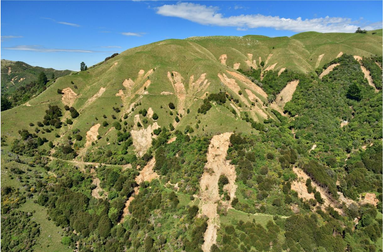
Figure 2.10 Shallow debris flows initiated in soil or colluvium in gully heads (tributary of Holyoake Stream, near Kaiterteri).
