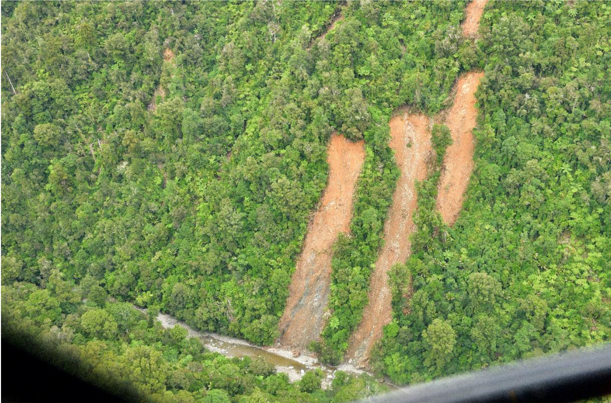
Figure 2.5 Examples of shallow soil and regolith landslides that occurred on open hillside faces and directly coupled to the stream channel (Upper Kaituna River).
