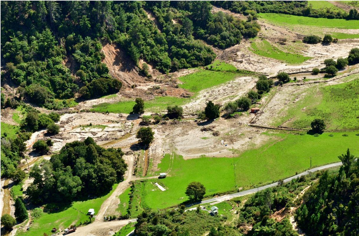
Figure 2.19 Examples of deeper-seated landslides in the Holyoake Stream catchment, Moss Rd, near Otuwhero Inlet.
