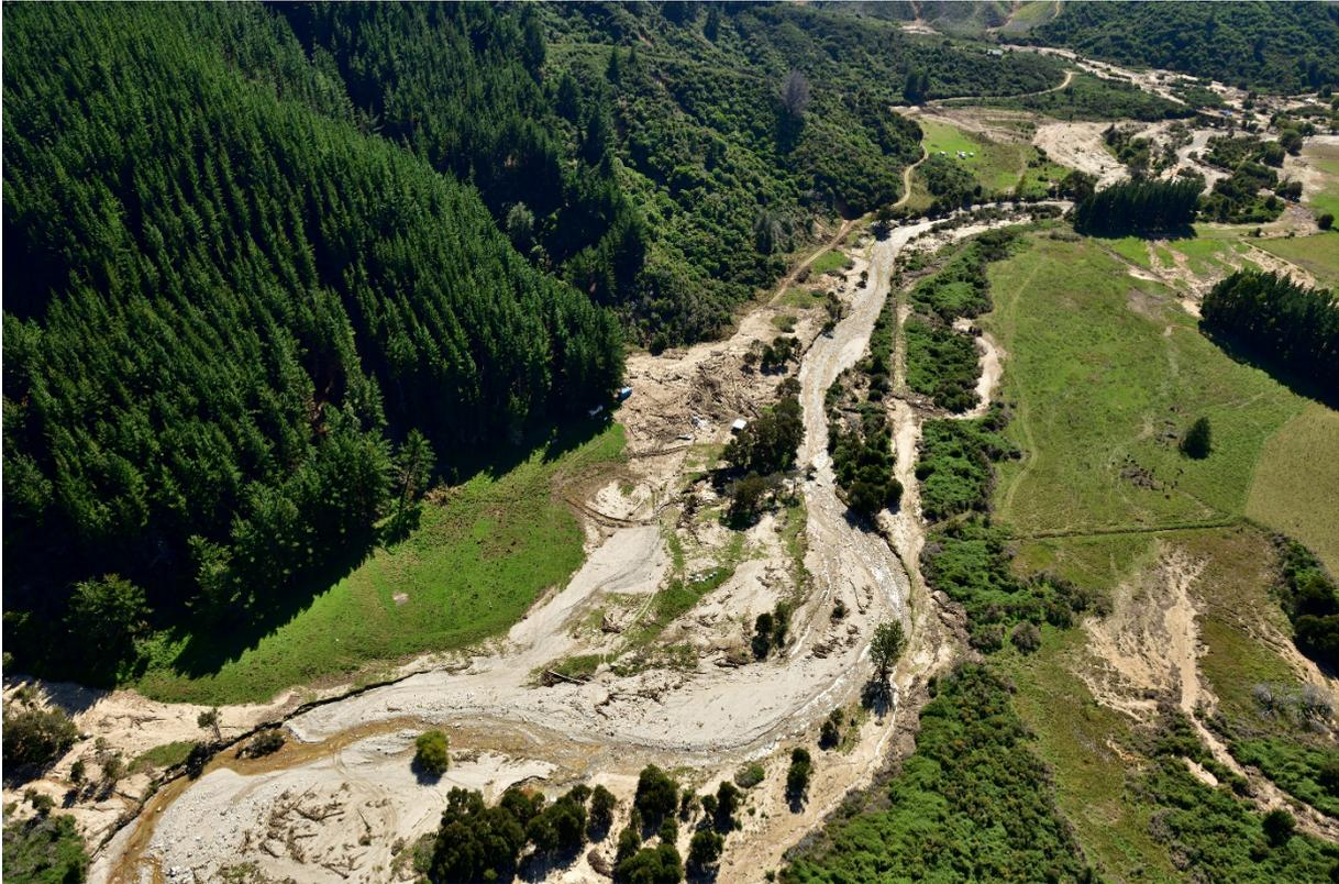
Figure 2.23 Debris flow deposit in the Otuwhero River near the upper end of the floodplain.
