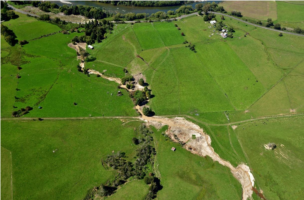
Figure 2.13 Channelised debris flow on the west bank of the Motueka river, near Pangatotara.
