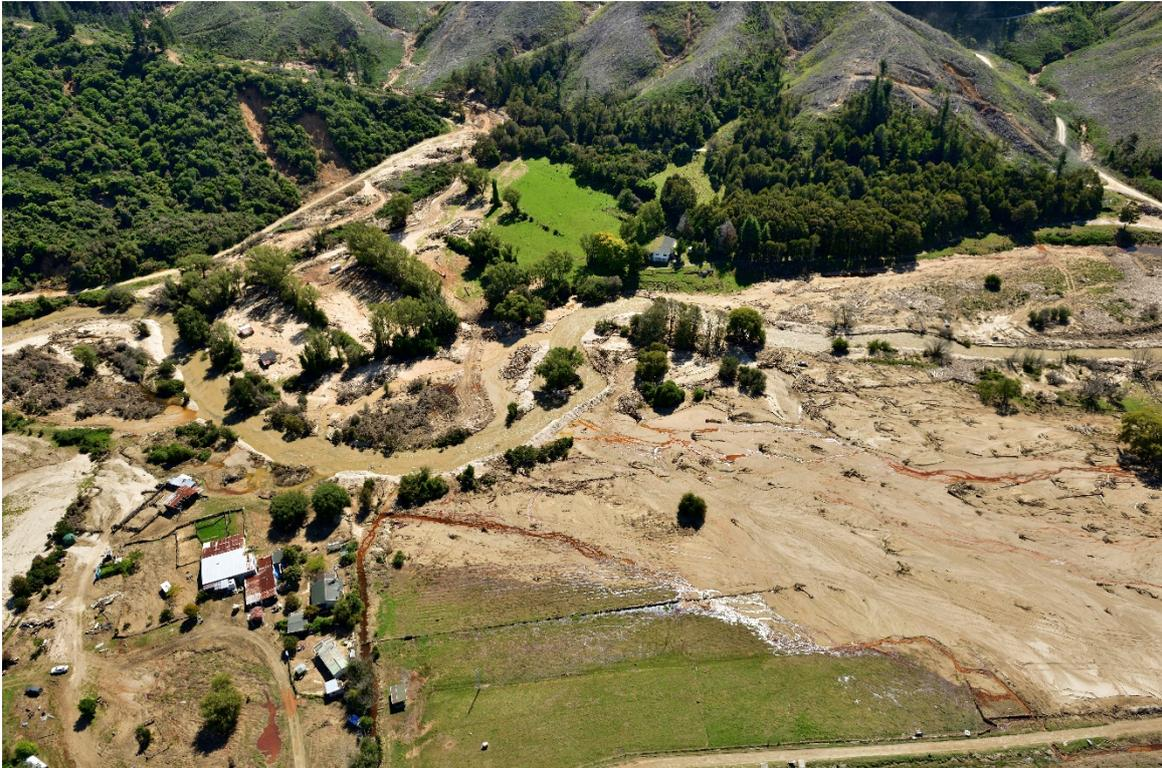
Figure 2.24 Debris flow deposit in the Otuwhero River catchment, at Otuwhero Valley Rd.
