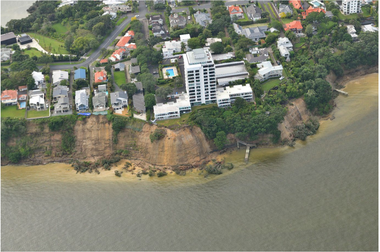
Figure A1.25 Photo 856_4494: Multiple shallow failures along the clifftops near Stanley Bay, Devonport. Failures are mainly in the weaker coverbeds (regolith/loess and volcanic soils).
