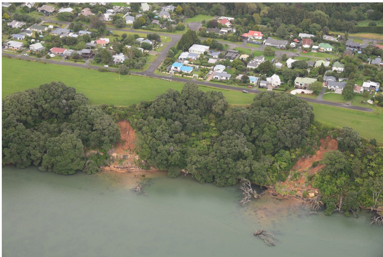
Figure A2.13 Photo DSC_9399: Small debris slides and avalanches in regenerating bush at Kauri Point, Tauranga Harbour.
