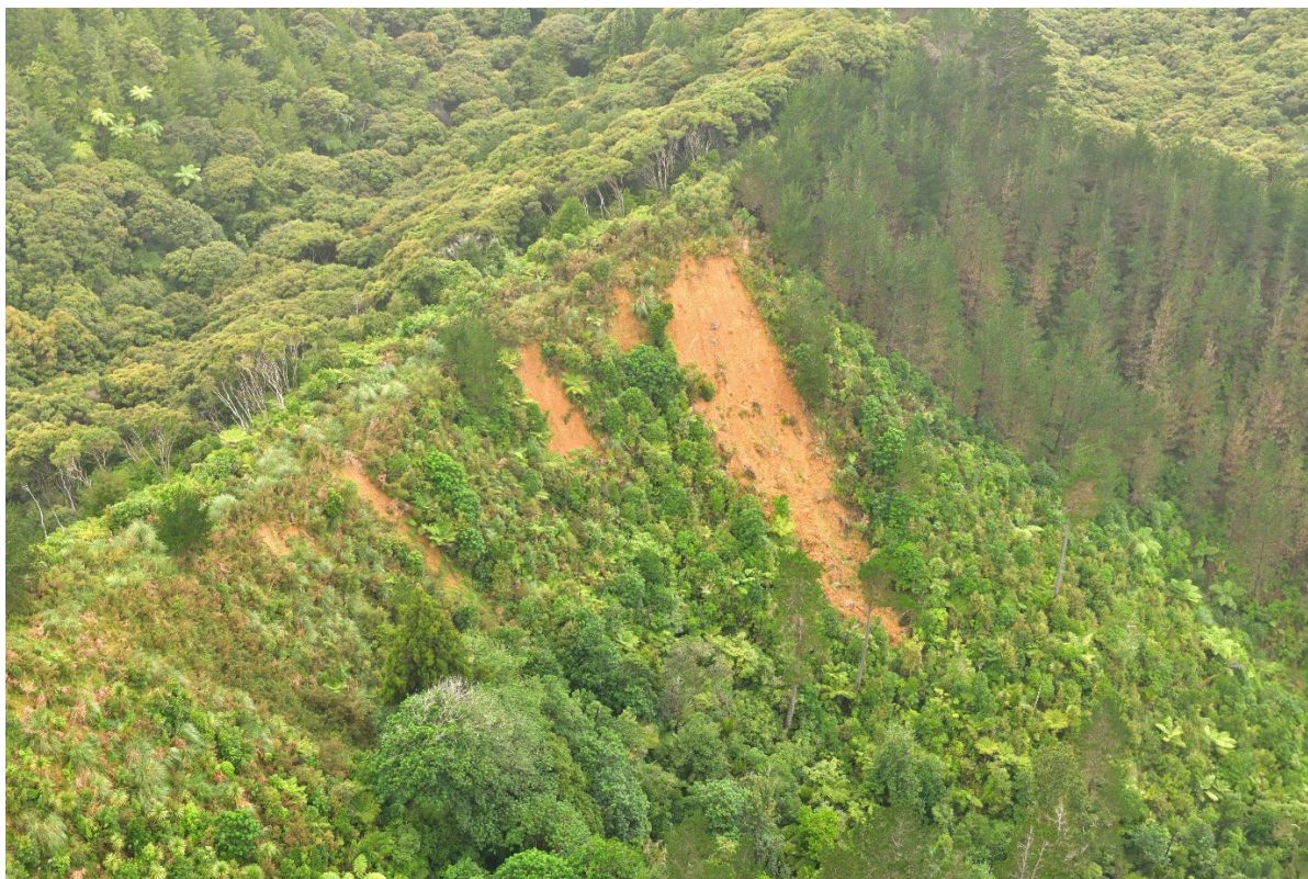
Figure A1.1 Photo 856_3829: Shallow landslides in regenerating forest/scrub inland from Langs Beach.
