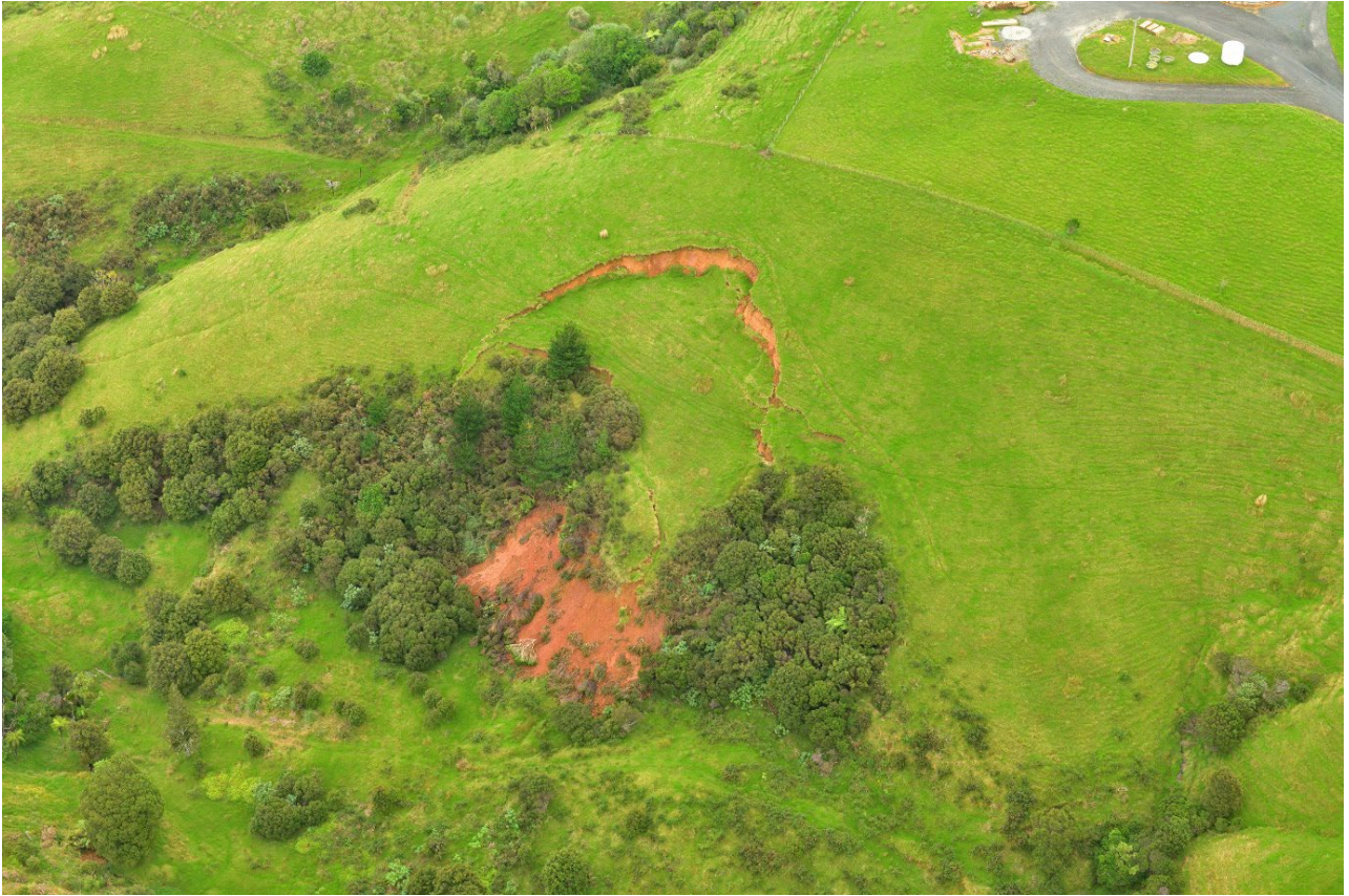
Figure A1.7 Photo 856_3928: Re-activation of deep-seated slump near Tāwharanui.
