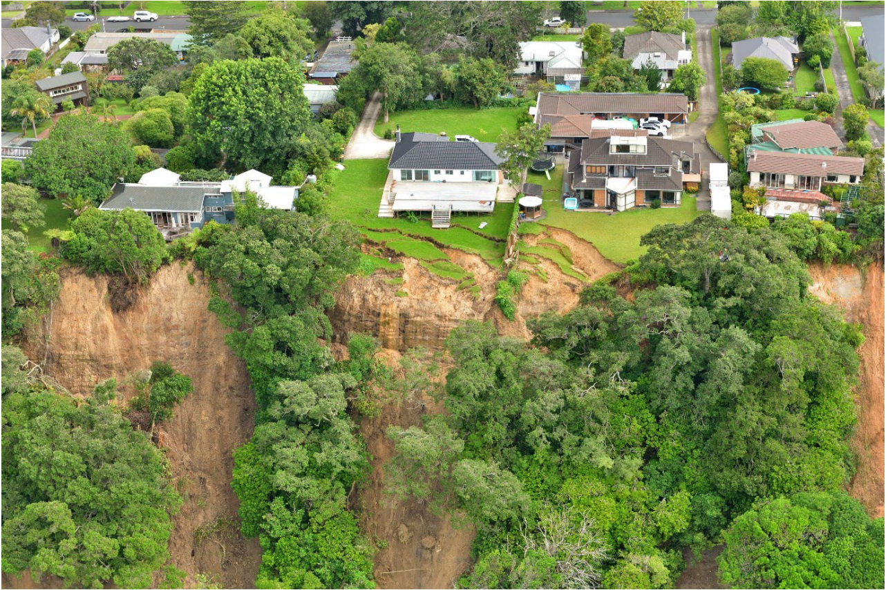
Figure A1.21 Photo 856_3066: Rotational slumping in cover beds above Waitematā Group rocks at Green Bay.
