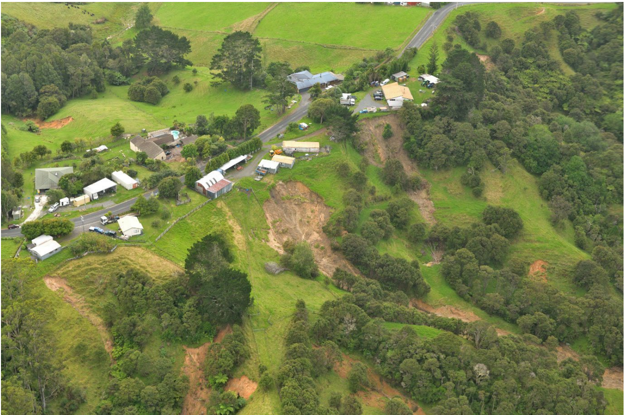
Figure A1.30 Photo 856_4359: Multiple collapses affecting properties at Albany Heights.
