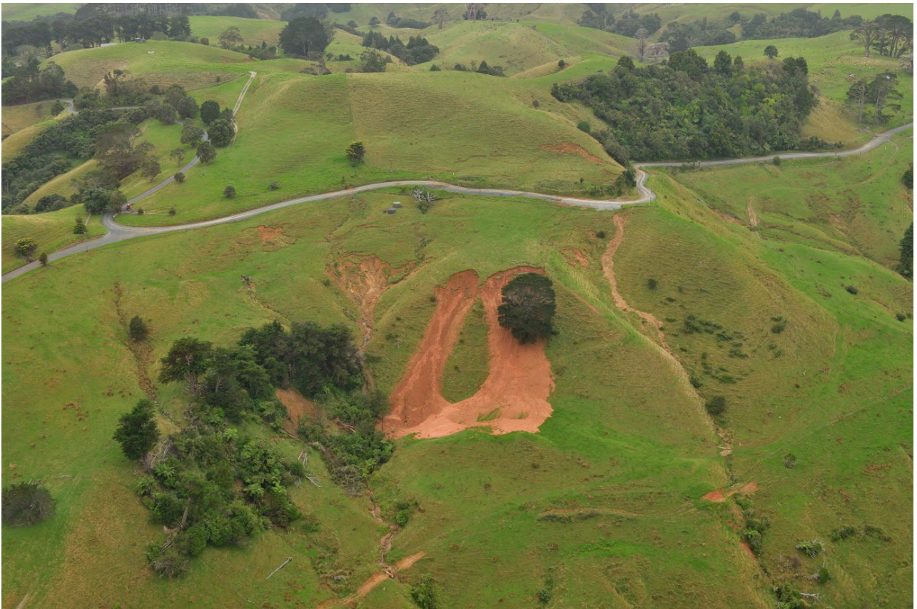
Figure A1.4 Photo 856_2523: Slumping and cracking in farmland and across Kaipara Hills Road. Note the fresh headscarp cracks in the paddock above the road.
