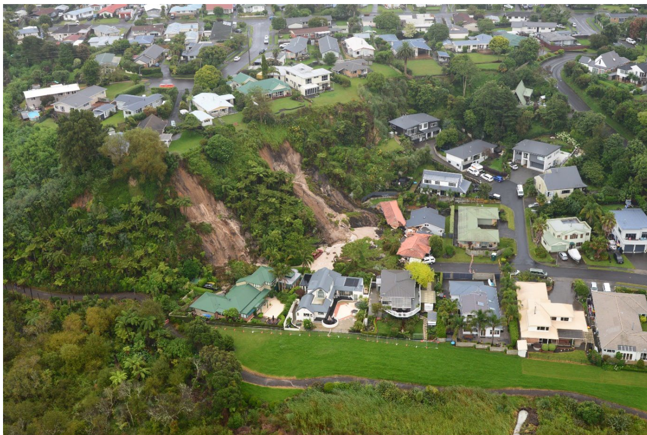
Figure A2.3 Photo DSC_9359: Two landslides in Welcome Bay (Tauranga) that significantly impacted houses, with one displacing a house by tens of metres.
