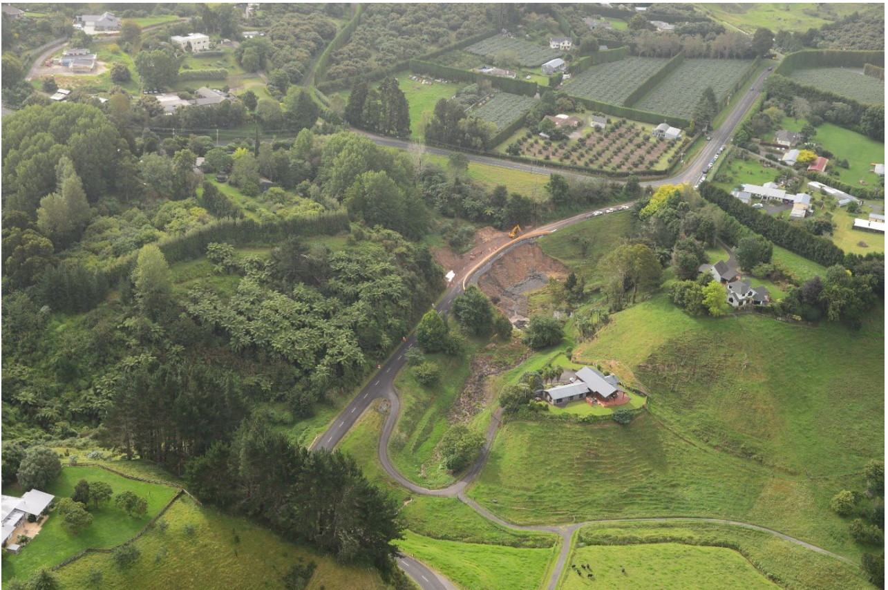
Figure A2.12 Photo DSC_9335: Landslide that damaged Wairoa Road (Wairoa, Tauranga Harbour), for which remedial works were underway.
