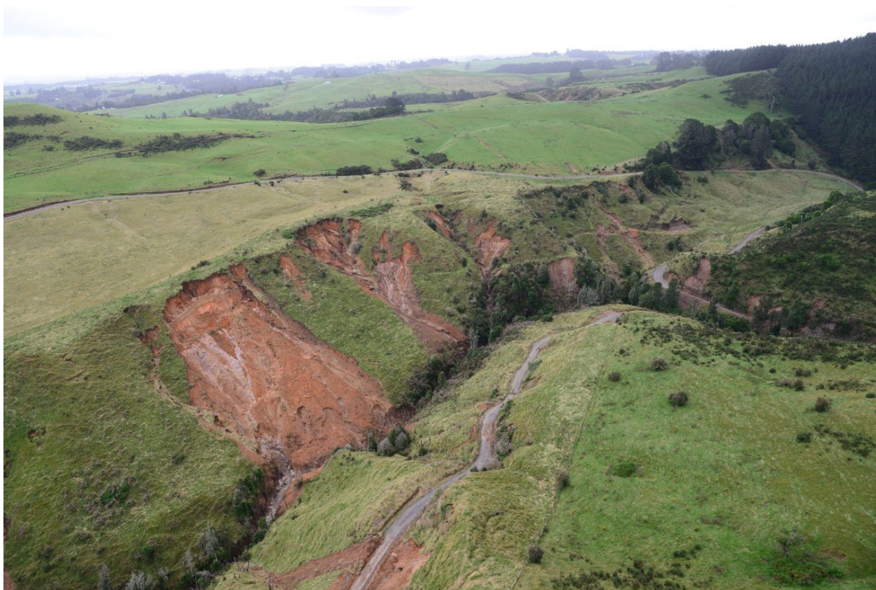
Figure A2.6 Photo DSC_9198: Examples southwest of Te Puke (Bay of Plenty) of landslides along valley shoulders (breaks in slope), which were particularly common in pasture and scrub.
