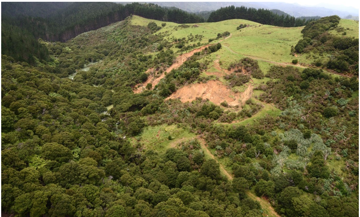
Figure A2.32 Photo DSC_9702: Rotational slide that has blocked the south branch of Waiwhango River, Coromandel, with a lake still present at the time of the photo. Cracks are also observed at the top of the hillslope, suggesting that a larger failure mass is involved.
