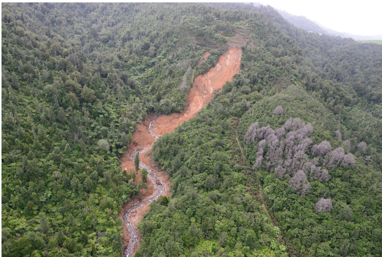
Figure A2.5 Photo DSC_9224: Large debris flow in regenerating forest southwest of Te Puke (Bay of Plenty).
