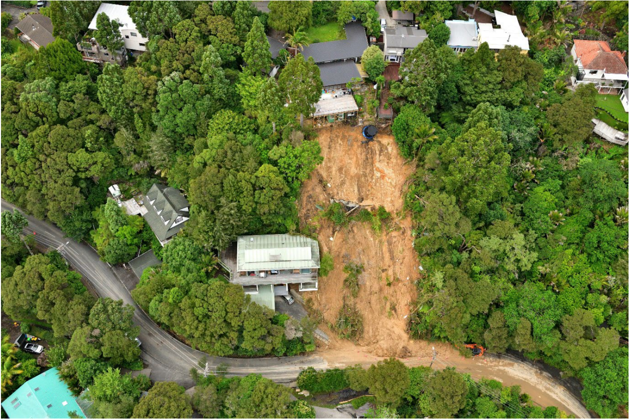
Figure A1.23 Photo 856_3022: Cliff collapse from beneath a house, onto another house and Wood Bay Road, Wood Bay, Titirangi.
