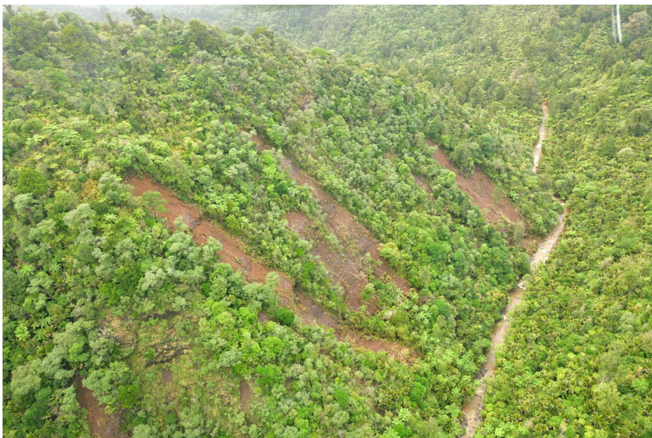
Figure A1.16 Photo 856_2953: Shallow debris slides in soil/regolith in the Waitākere ranges.
