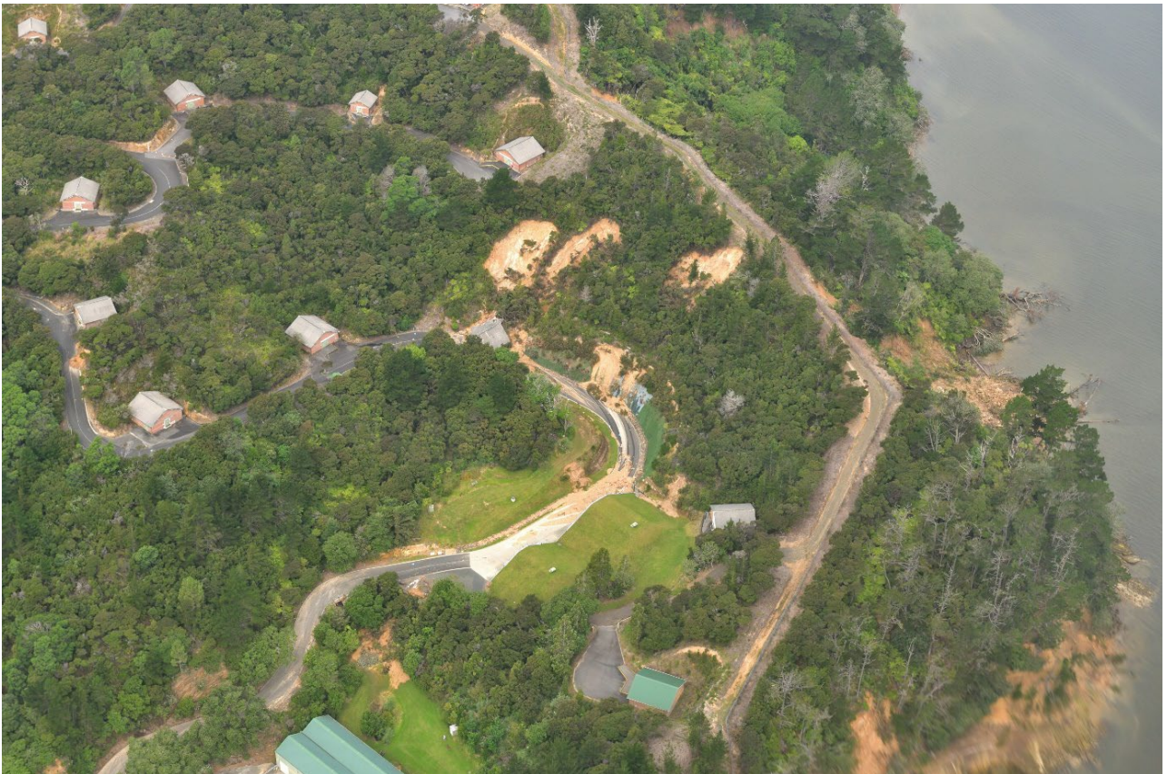
Figure A1.28 Photo 856_4440: Multiple small failures at Onetaunga Bay, Chatswood. Note that one building has been pushed off its foundations and is now on the road.
