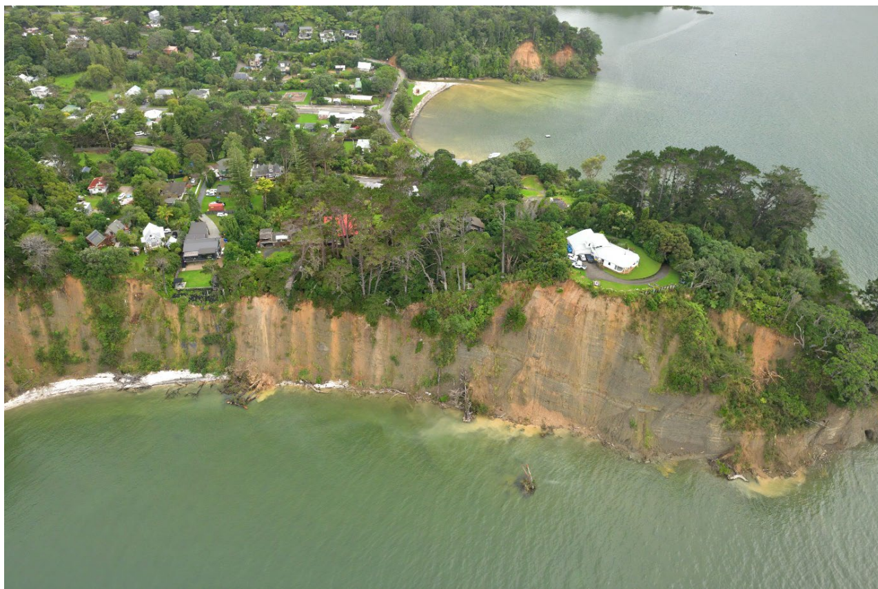
Figure A1.19 Photo 856_2979: Multiple collapses along the clifftops near Tokoroa Point. The failures are mainly in the weaker coverbeds (regolith/loess and volcanic soils) that overlie Waitematā Group rocks.
