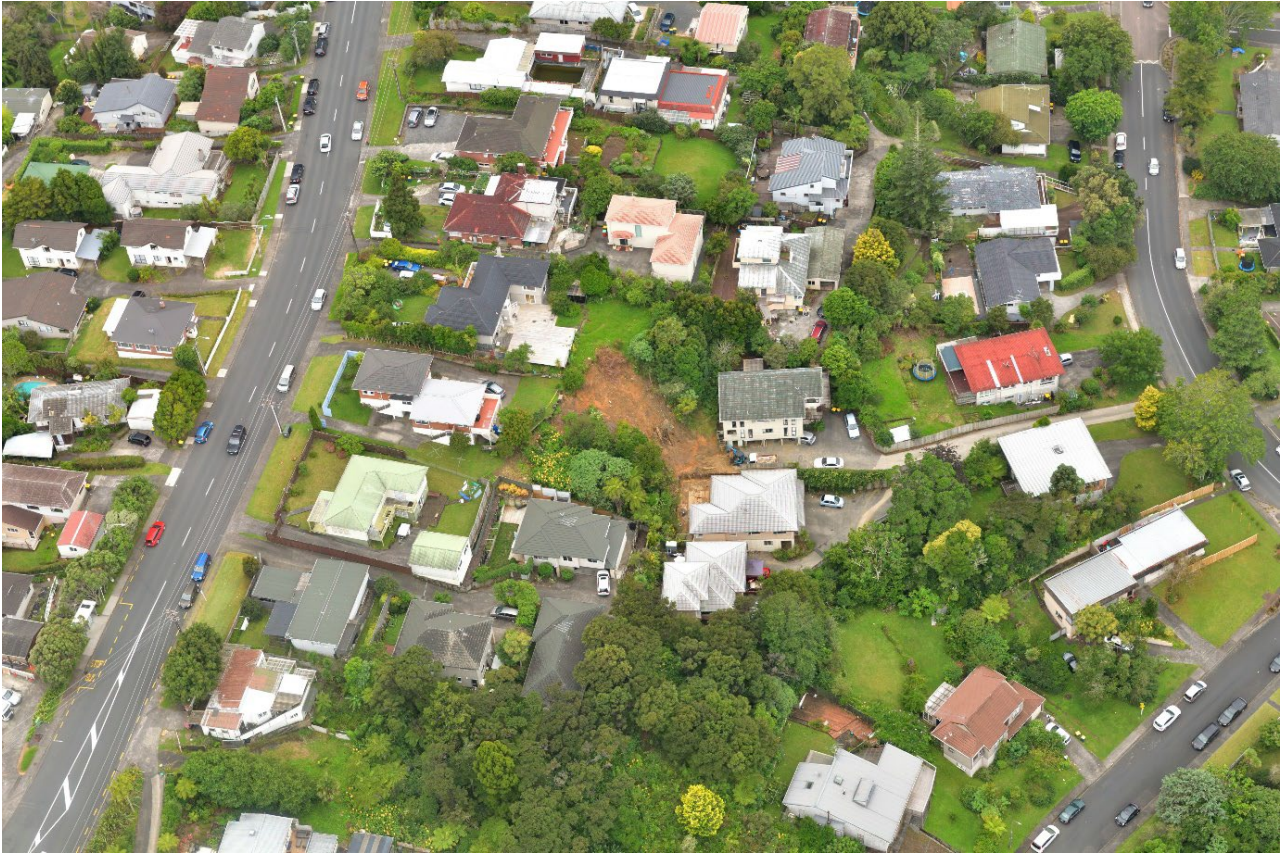
Figure A1.29 Photo 856_4028: Collapse of a property at Glenfield.
