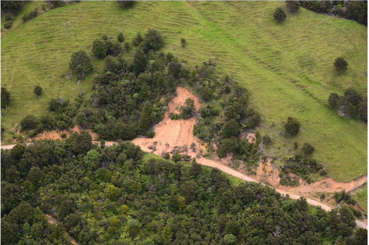
Figure A2.21 Photo DSC_9464: Debris slides and falls were common along rural roads, driveways and farm tracks, such as in this example from Waiomu, Coromandel Range.
