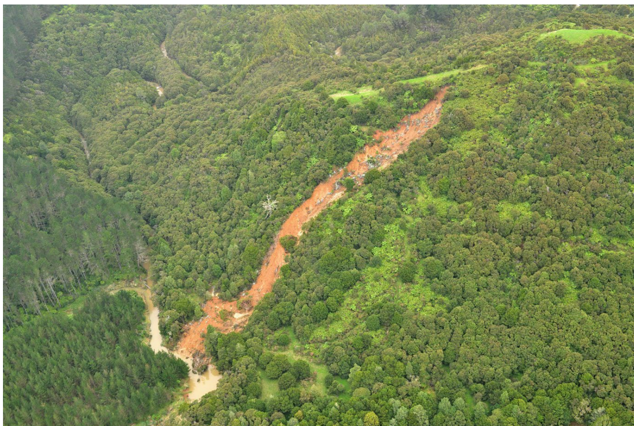
Figure A1.6 Photo 856_3861: Debris avalanche partially blocking Waiwhiu Stream, east of Wellsford.
