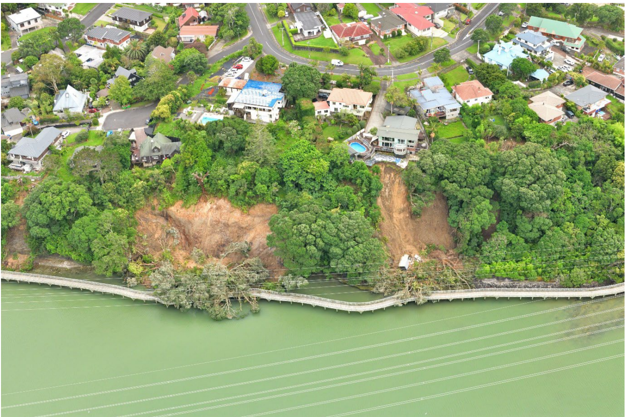
Figure A1.22 Photo 856_3150: Collapse of coastal cliffs undermining property and houses at Hillsborough.
