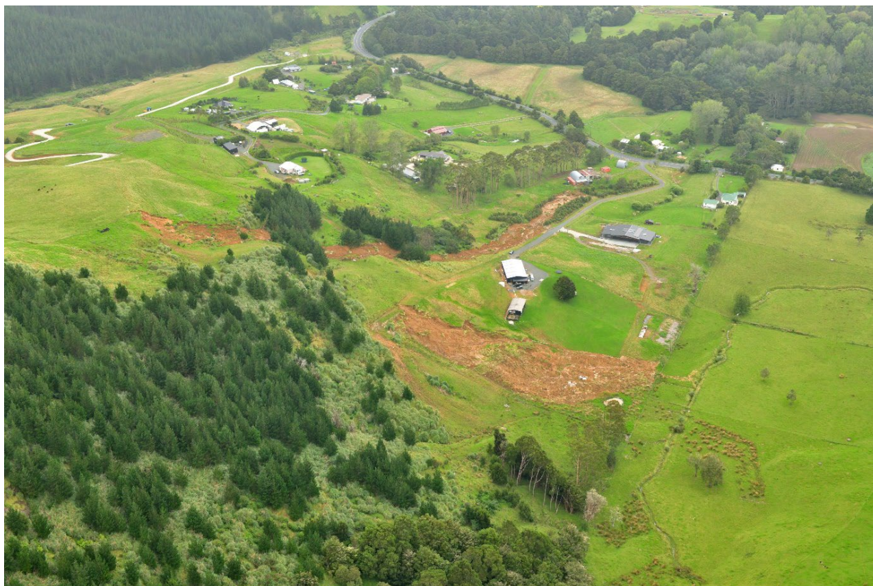
Figure A1.5 Photo 856_3888: Multiple slides and slumps at Whangaripo, east of Wellsford.
