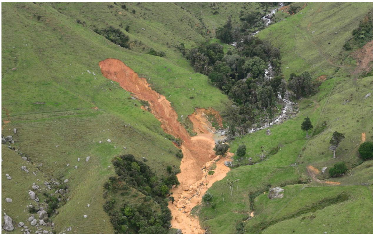
Figure A2.34 Photo DSC_9621: Slope failures were prevalent in the Te Mata Group sedimentary rock and overlying regolith in Coromandel. Some of these, such as the example here from Ohinewai Stream, Moehau Range, transitioned downslope into debris flows.
