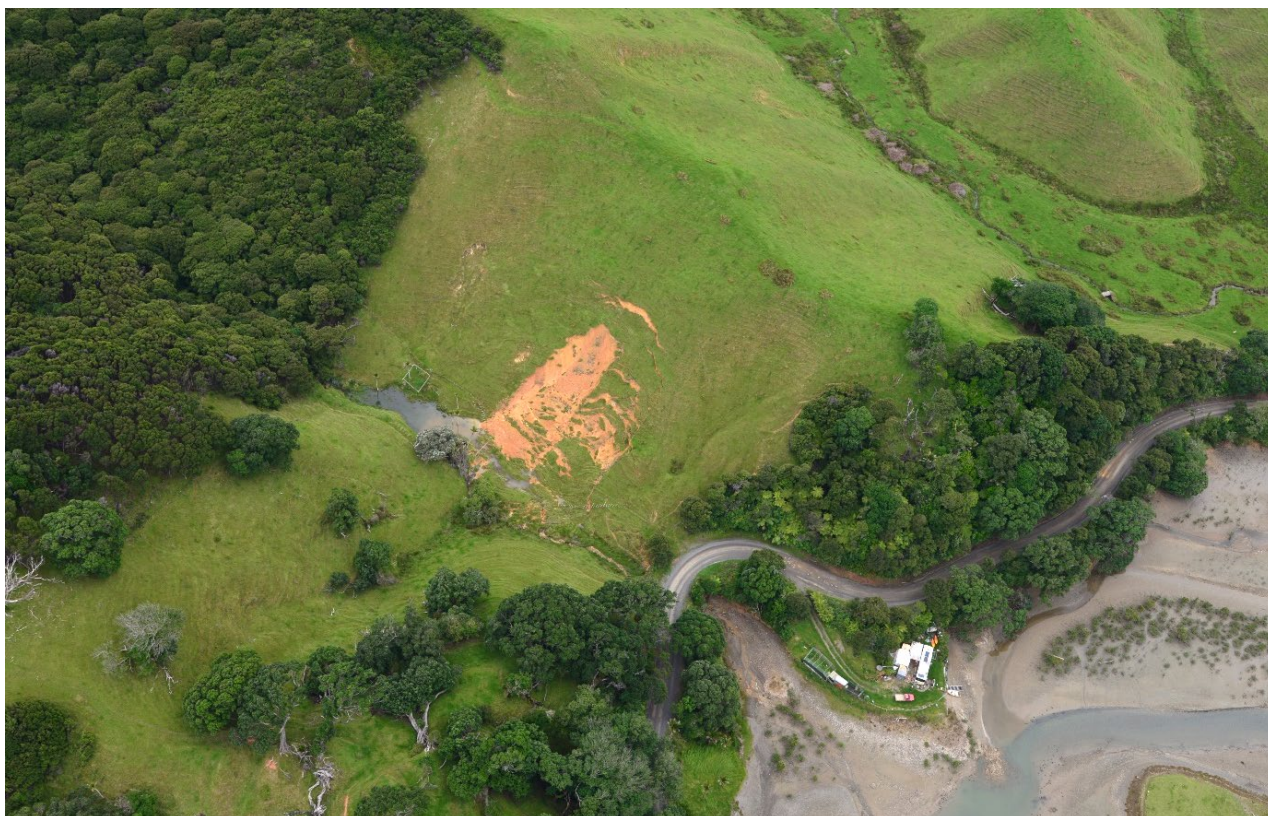
Figure A2.33 Photo DSC_9652: A slide in regolith/soil has blocked a small stream, creating a small lake upstream of a road and small dwelling, with potential for further displacement and enlargement of the landslide mass indicated by cracks in the hillslope above the freshly exposed debris. Port Jackson Road, Waiaro.
