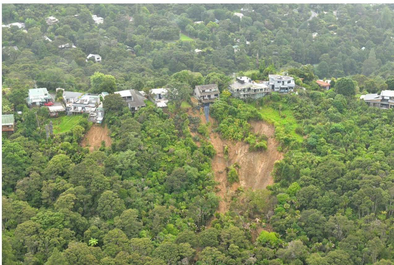
Figure A1.18 Photo 856_2969: Collapse of regolith from volcaniclastic rocks (Nihotupu Formation) beneath houses at Laingholm.
