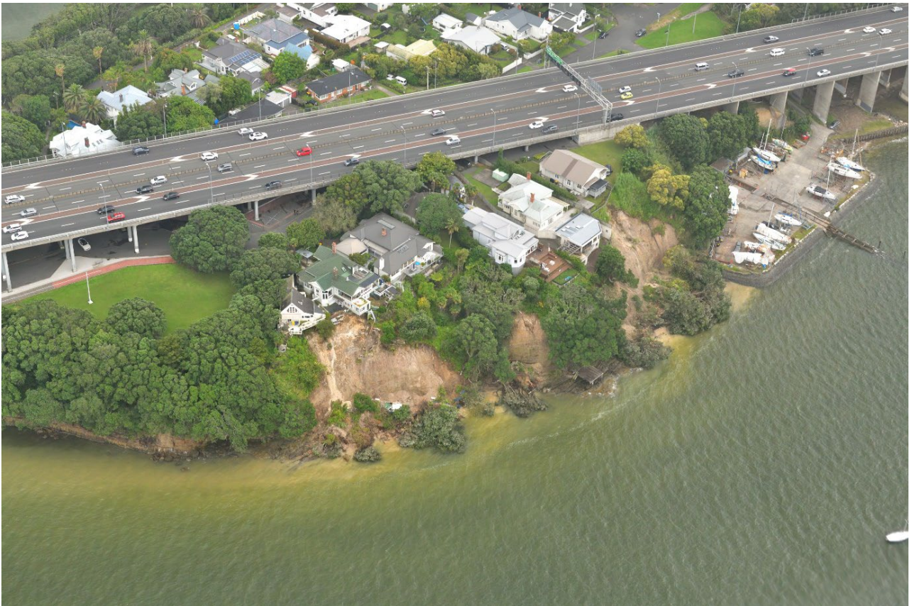
Figure A1.24 Photo 856_3249: Coastal cliff collapses at Stokes Point, undermining houses.
