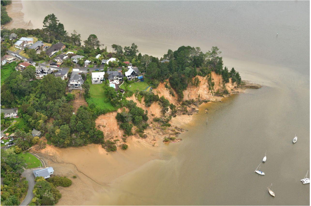
Figure A1.27 Photo 856_4392: Multiple failures in weathered East Coast Bays Formation, Greenhithe.
