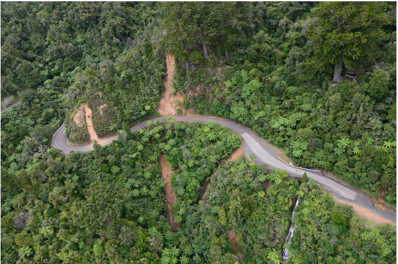
Figure A2.22 Photo DSC_9501: Examples of failures above and below the Tapu Coroglen Road, Coromandel Range.
