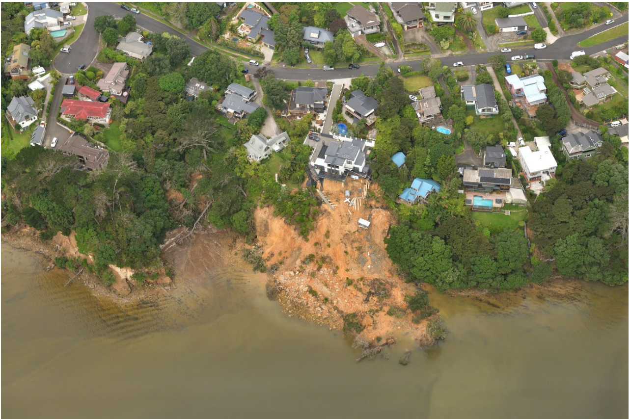
Figure A1.26 Photo 856_4428: Deep-seated collapse of weathered Miocene East Coast Bays Formation, undermining a house near Beach Haven, Birkenhead.
