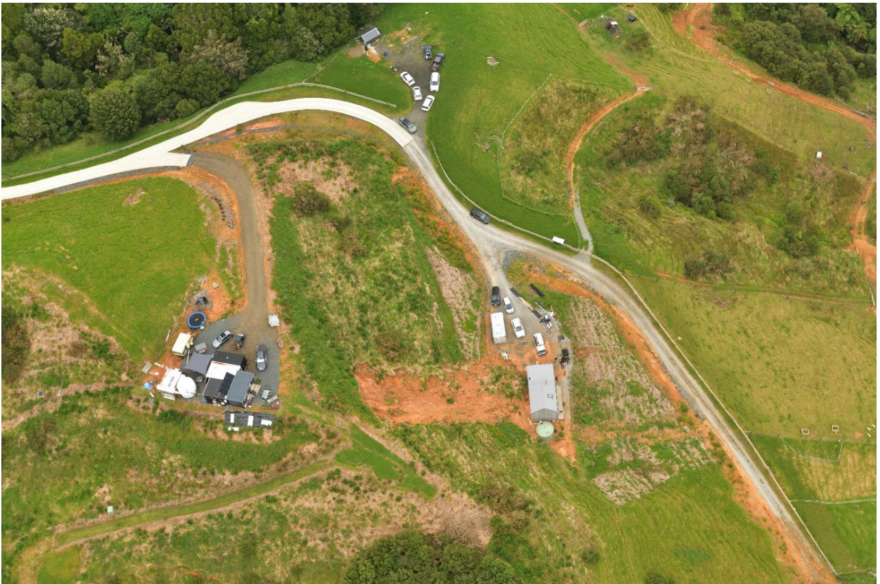
Figure A1.8 Photo 856_3534: Small debris avalanche in developed farmland near Pūhoi, impacting a recently built house.
