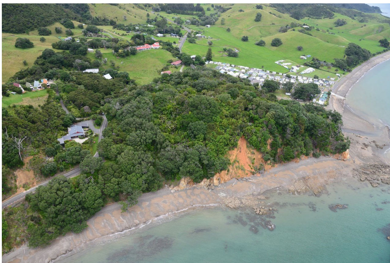
Figure A2.30 Photo DSC_9688: Coastal landslide and small failure onto Colville Road, Papaaroa.
