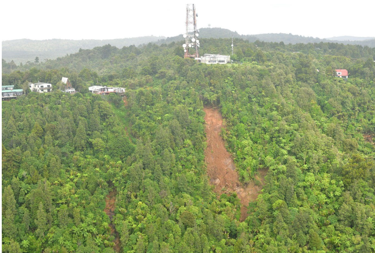
Figure A1.17 Photo 856_3317: Shallow landslides in soil/regolith below Parkinsons Lookout, Waiatarua.
