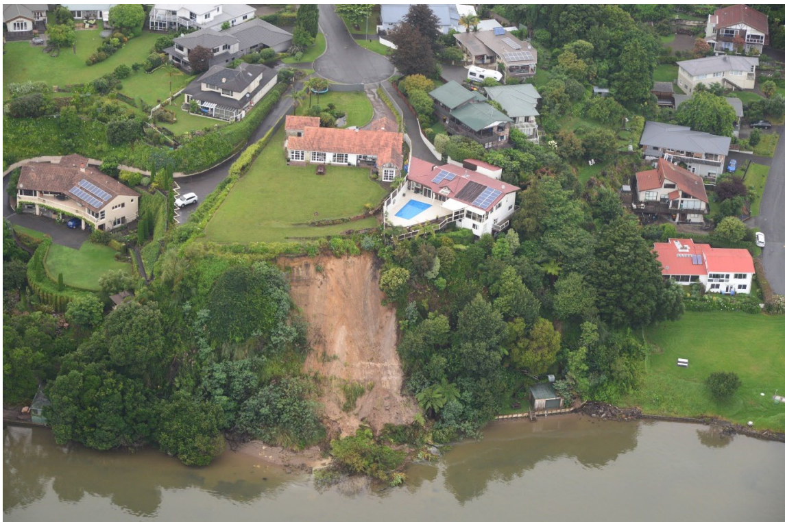
Figure A2.2 Photo DSC_9392: Example of landslide from steep coastal slope of Waimapu Estuary (Tauranga).
