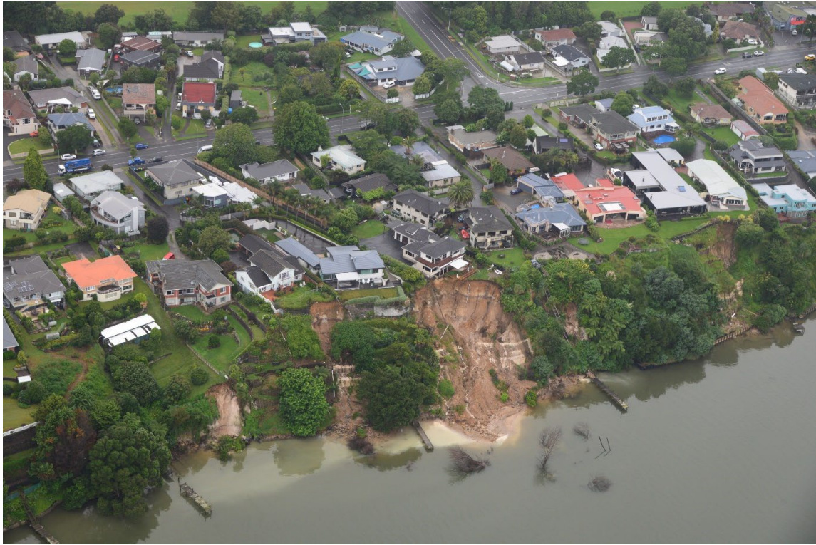
Figure A2.1 Photo DSC_9385: Landslides along steep coastal slopes and cliffs of Waimapu Estuary (Tauranga), some of which have affected residential properties.
