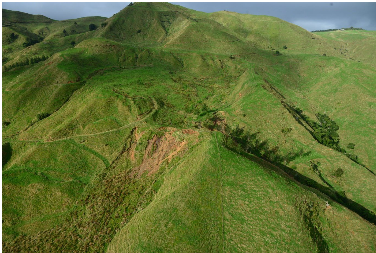
Figure A2.14 Photo DSC_9955: Example of small, shallow soil avalanches/flows on hill country terrain (in pasture), near Te Aroha, Kaimai Range.
