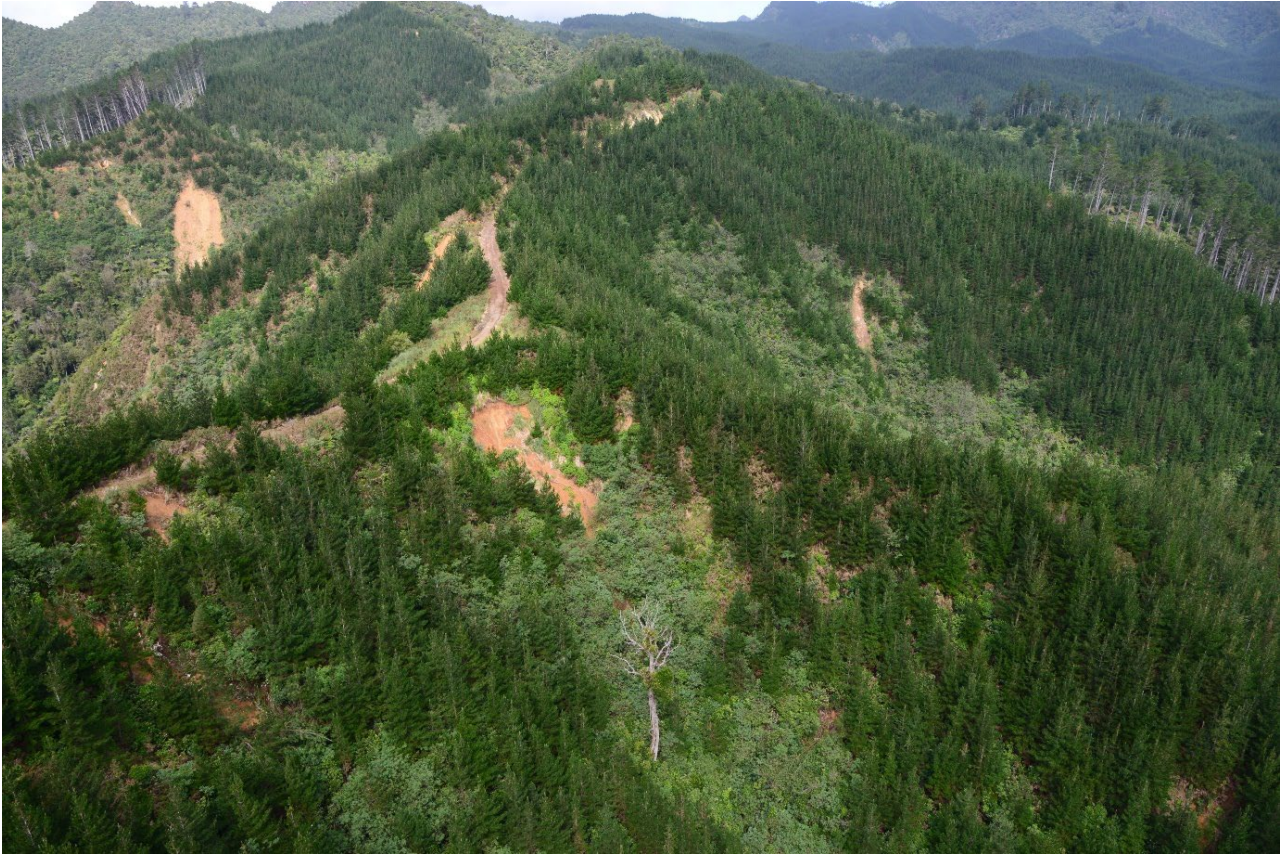
Figure A2.27 Photo DSC_9790: Landslides were common in forestry areas, particular in young or recently cut-over slopes. The photo is taken in a forestry block between Mātāwai and Purunui streams, Coromandel.
