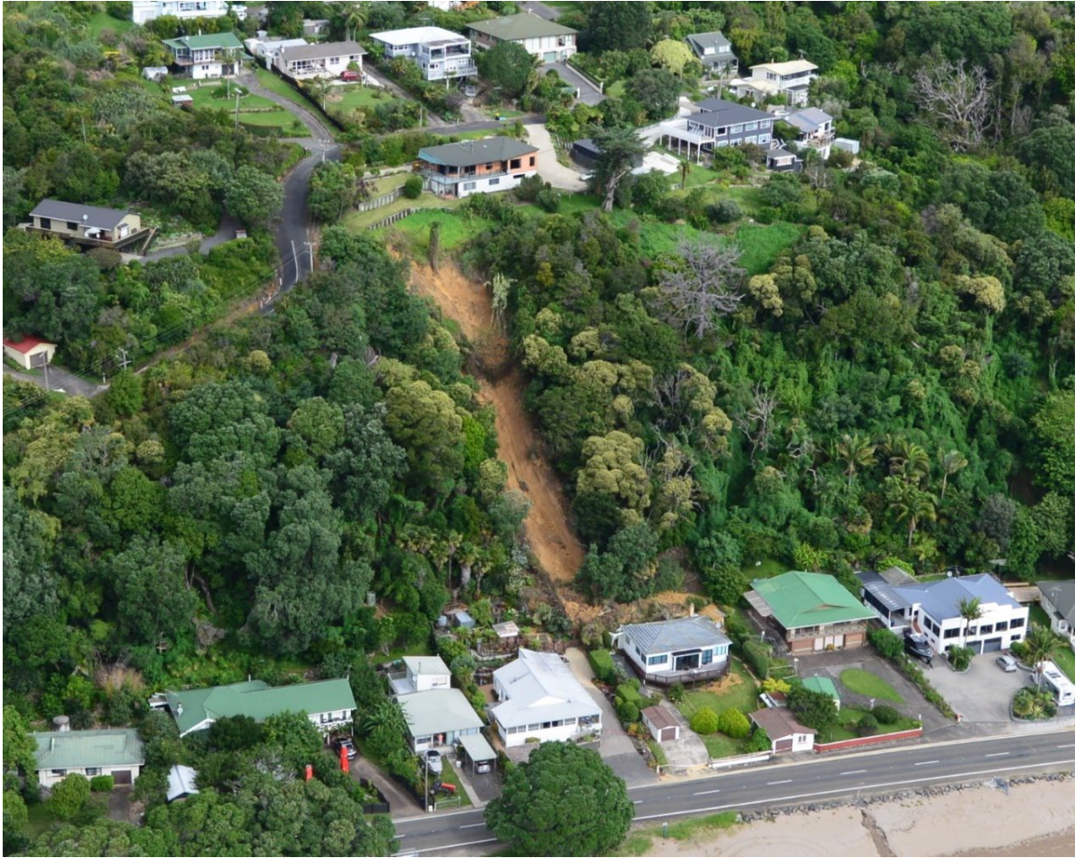
Figure A2.19 Photo DSC_9913b: Debris slide that transitioned into a flow and impacted a house in Thornton Bay, Coromandel Range.
