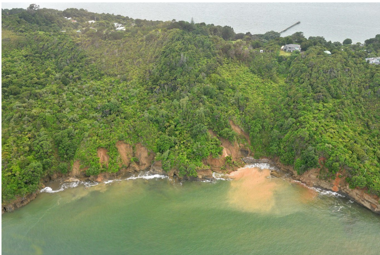
Figure A1.15 Photo 856_2910: Collapse of volcaniclastic rocks along the coastline near Cornwallis.
