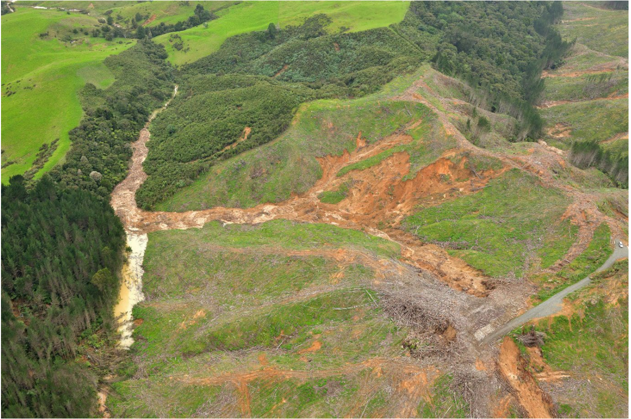
Figure A1.9 Photo 856_3570: Debris avalanches entraining forestry slash and forming a small dam in a gully that feeds into Hikauae Creek near Cook Road, just north of Pūhoi, Auckland. The stream drains towards State Highway 1.
