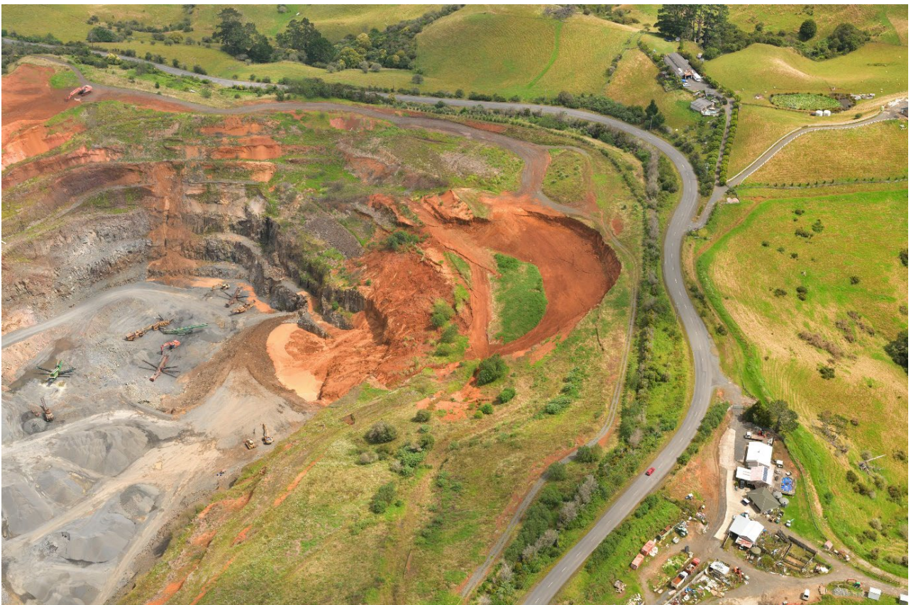
Figure A1.32 Photo 856_4126: Collapse in a quarry near Pōkeno, likely to be a re-activation of an earlier slump.
