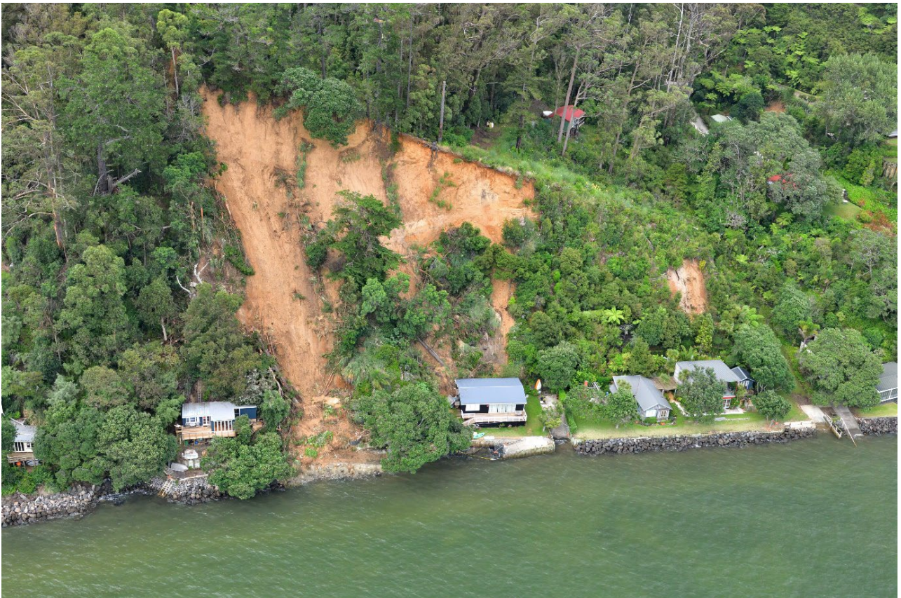
Figure A1.14 Photo 856_2833: Coastal cliff collapse at Ōrua Bay, northern Āwhitu Peninsula, where debris impacted a bach (now removed) trapping three occupants.
