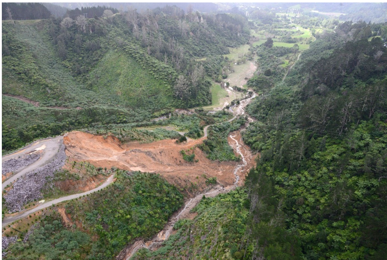
Figure A2.4 Photo DSC_9154: A debris flow from a forestry slope that has choked a stream with sediment and woody debris, in the Waitao catchment (Tauranga).
