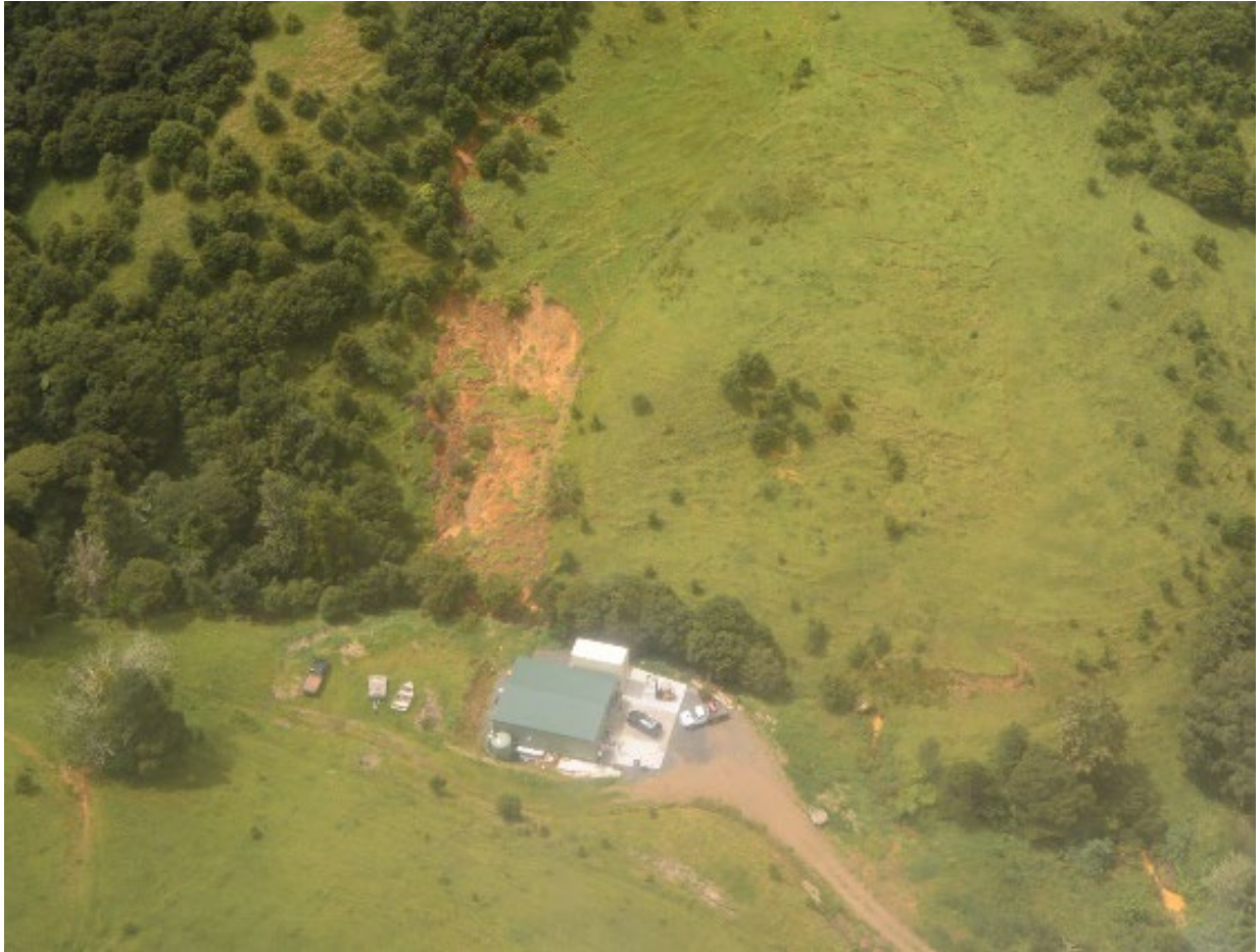
Figure A2.31 Photo DSC_9711: An incipient failure (note cracks and deformed ground visible above and right of the fresh landslide scar) situated near a building; Kikowhakarere Bay, Coromandel.
