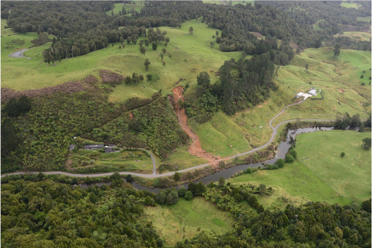
Figure A2.9 Photo DSC_9284: Example of small debris flow onto a vehicle track, southern Kaimai Range (Bay of Plenty).
