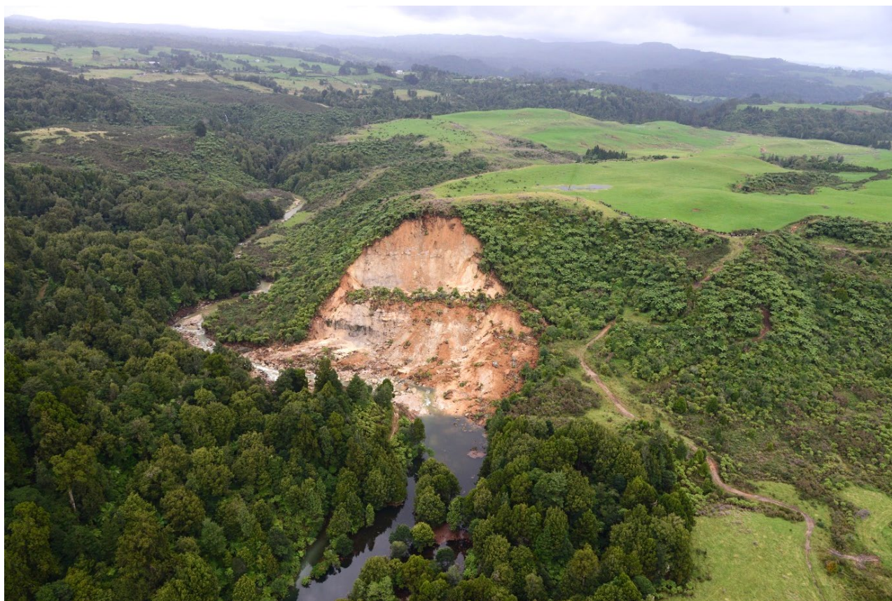
Figure A2.8 Photo DSC_9274: A large rotational landslide from outside of a bend in the of Kaukaumoutiti Stream in southern Kaimai Range (Bay of Plenty), and the impounding of the river by the debris dam.
