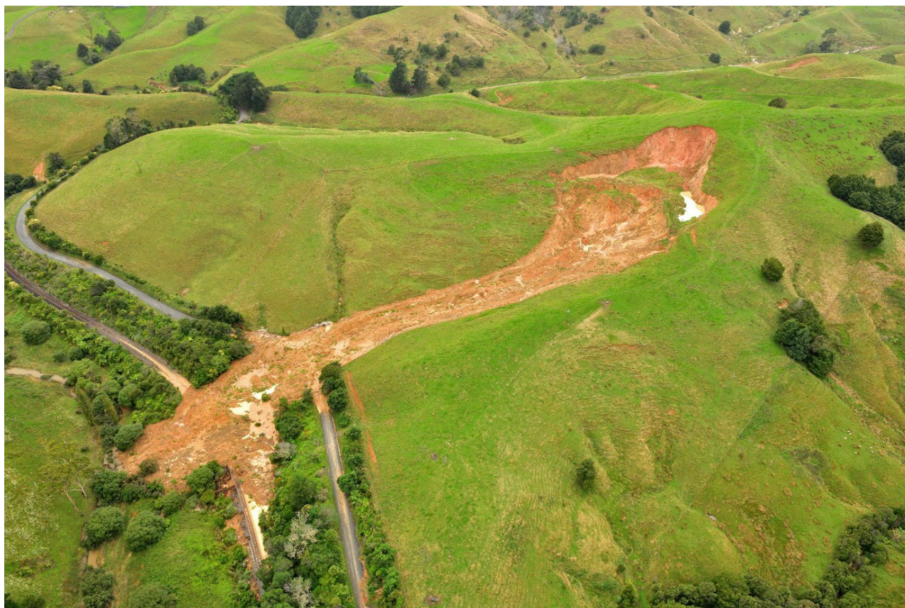
Figure A1.12 Photo 856_2616: Large debris avalanche in farmland near Tāhekeroa, sending debris over the North Auckland Line railway and Tāhekeroa Road.
