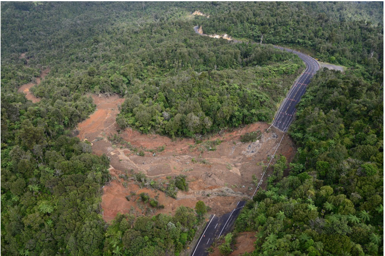
Figure A2.16 Photo DSC_9444: Large debris flow sourced from a gully-head failure that has undermined State Highway 25A, Coromandel Peninsula. The debris flow travelled 1.5 km into Kirikiri Stream.
