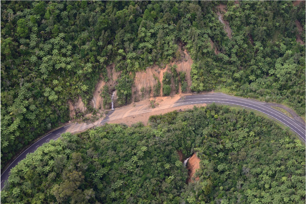
Figure A2.15 Photo DSC_9428: Shallow soil and vegetation failures onto State Highway 25A, Neavesville, Coromandel Peninsula.
